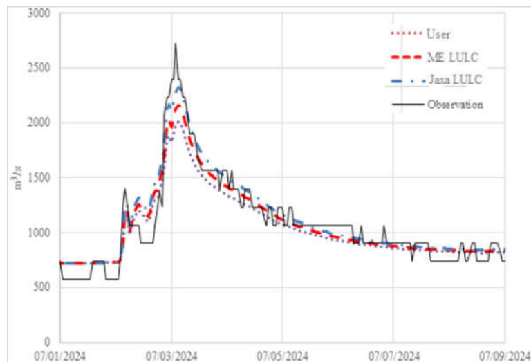
Figure 6: Verification of Tuyen Quang reservoir inflow in 07/2024
