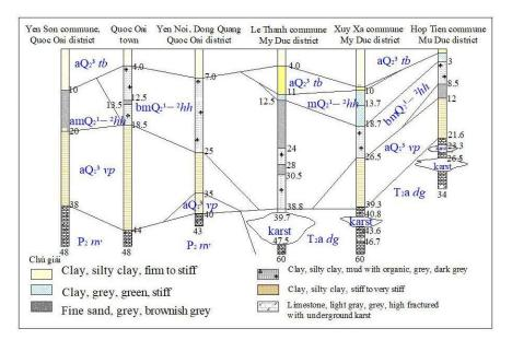
Figure 4: Combining succession of strata of ground collapse position in the Western, Southwestern areas of Hanoi city [2, 5]
