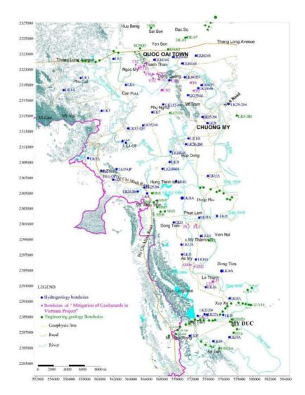
*Figure 1: Locations of boreholes in the Western and Southwestern areas of Hanoi city [2]* In the plains, limestone is exposed commune (from -11 m to -15 m). In other
